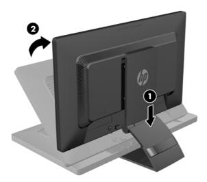
NOTE: When the monitor is unfolded for the first time, the display head is locked from adjusting to a full-height position. To adjust the display head to full height, press down on the display head to unlock it then pull up on the display head to raise it to the full-height position. Refer to step 3 in <a href="Adjusting the Monitor on page 13">Adjusting the Monitor on page 13</a>.
