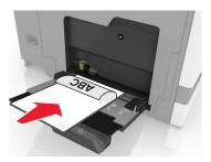
• Load envelopes with the flap side up and against the left side of the paper guide. Load European envelopes with the flap side up and entering the printer first.
