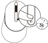
2. The third-bluetooth connection light (3\*) starts blinking to confirm the pairing mode is enabled.
